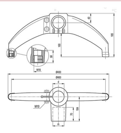
d (inch) = 1 1/2 Gas d1 (inch) = 1 1/4 Gas d1 (mm) = 42.4 d mm = 48.3 Weight (g) = 710
